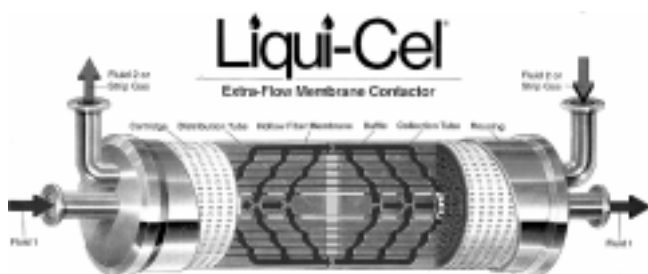
Fig. 4. Schematic representation of the structure of Liqui-Cel liquid membrane contractor.
